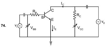
In the figure, given that  $V_{BB}$  supply can vary from 0 to 5.0 V,  $V_{CC}$  = 5 V,  $\beta_{dc}$  = 200,  $R_B$  = 100 k $\Omega$ ,  $R_C$  = 1 k $\Omega$  and  $V_{BE}$  = 1.0 V. The minimum base current and the input voltage at which the transistor will go to saturation, will be, respectively:
